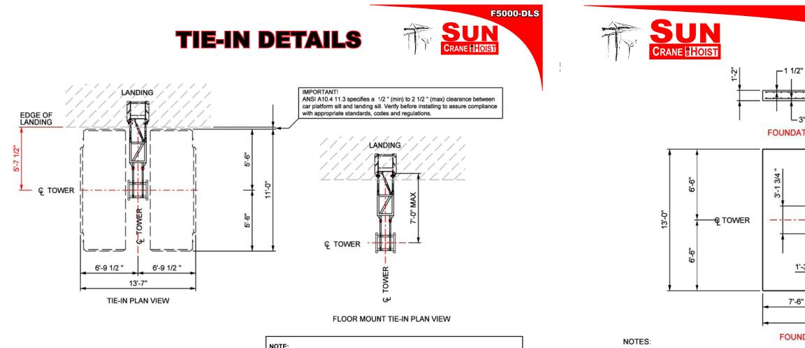
Distance above are for a typical 5 tir-in. Alternate anchoring methods are available.
